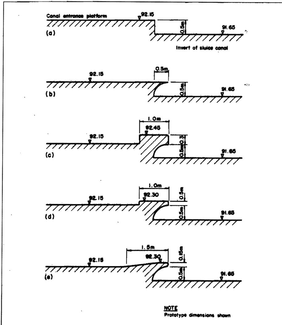
Figure 6 Skimming weir details for different models
