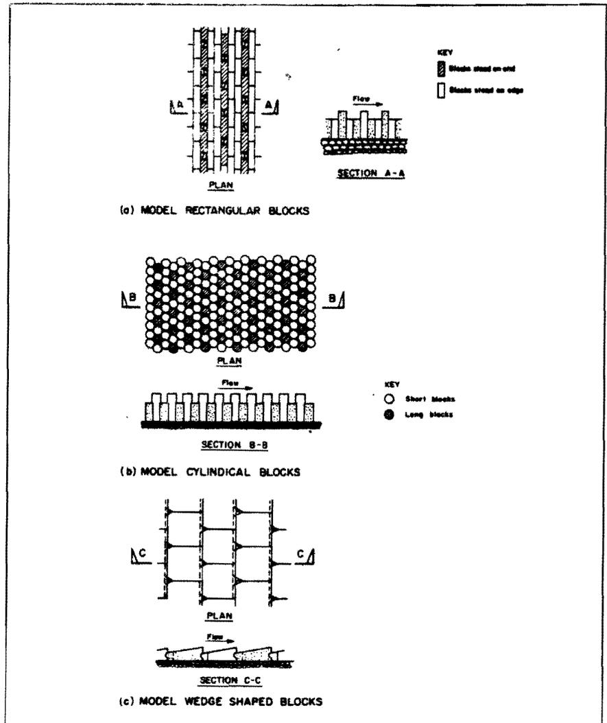
Figure 7 Model blocks for concrete block weirs
