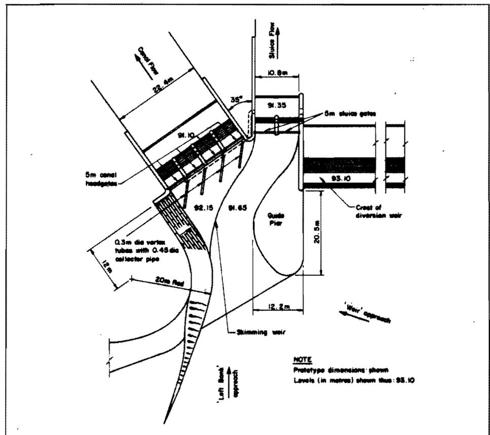
Figure 5 General layout of headworks for model tests
