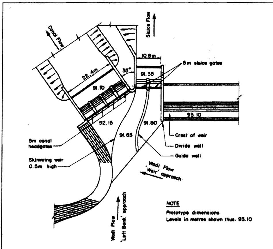
Figure 4 Preliminary layout of headworks for model tests
