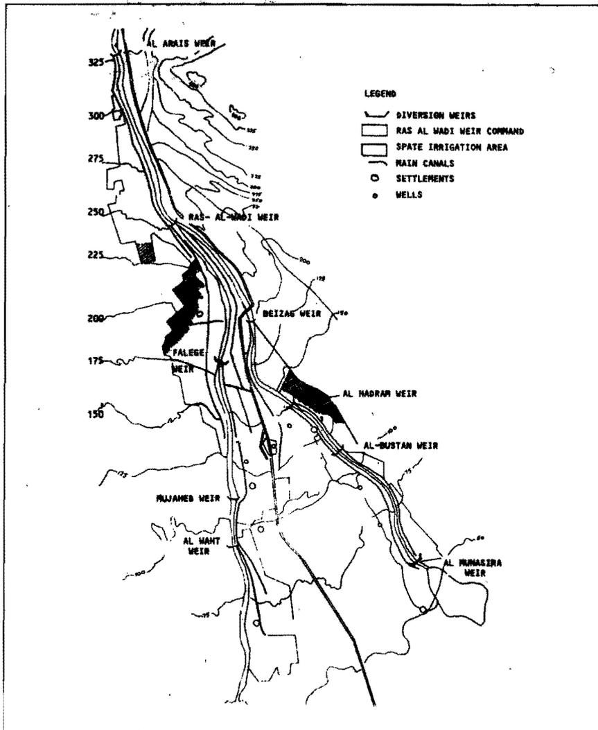
Figure 1 Layout of diversion weirs on Wadi Tuban
