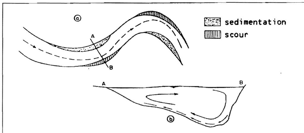
Figure 2 Scour and sedimentation in meander curve
