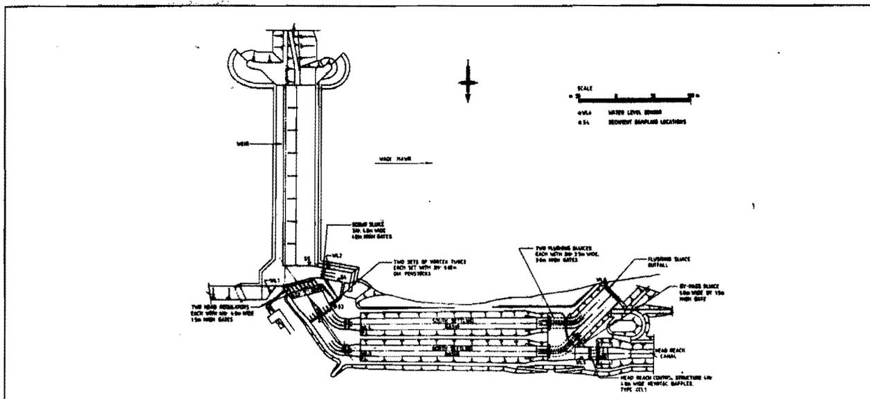
efficiency; at 50 m<sup>3</sup>/s, a 25 percent increase in abstraction capacity, the diversion efficiency increases only 2 percent from 88 percent to 90 percent. An analysis of costs showed a similar pattern. Thus the canal headworks capacity was set at 40 m<sup>3</sup>/s, slightly in excess of that required to provide an average duty of 2 l/s per hectare over the estimated net irrigable area of 18 800 ha.
